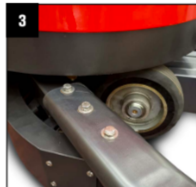
3 Screw and tighten the three M8 screws
