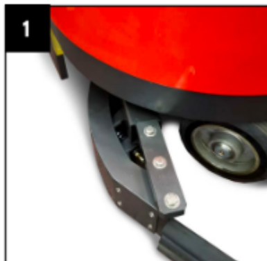
1 Unscrew the three M8 screws
