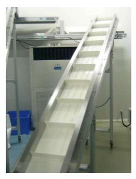
The STEP LMM-TSC01 is a transport conveyor system with customizable transport speed. Customizable according to customer specification to meet the production demands. It is ideal with most production line as a transporting conveyor to complete complex lines.
