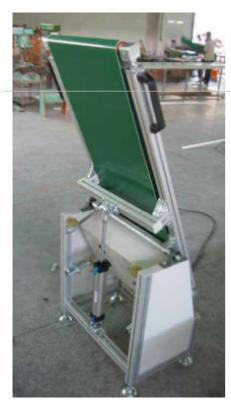
Made with light aluminum frames and is suitable for electronics and light production industry. The conveyor build is fully customizable to meet the customer specifications.
