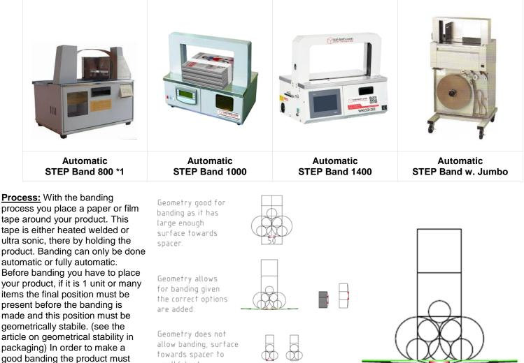
banding spacer/surface, so when the tape is tightened it can release. You can band both hard and soft products within limitations. The area towards the spacer surface must be above 50mm and flat. Banding is great for product that have little strength, using banding you can use zero tension just placing he tape around your product and you can tension up to about 18 kg depending of machine.
