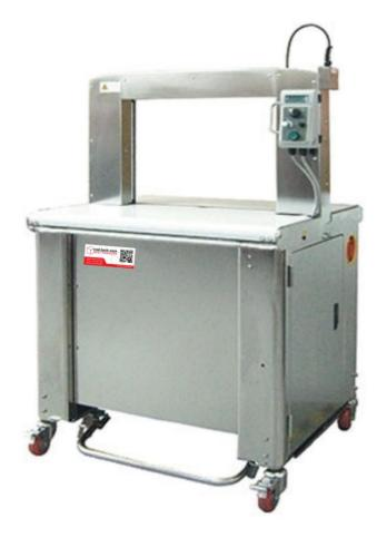
The STEP TP-702RSS is a high-speed automatic strapping machine with a stainless steel frame. It delivers dependable high speed performance for tiny or round package applications and is suited for damp working environments such as meat, seafood, poultry, and agricultural processing operations.
