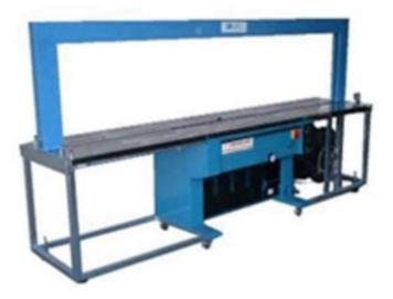
Automatic strapping machine, produced in Taiwan and project built in Denmark.
