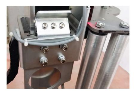
Observe the direction of the aggregate mounted where the M6x16mm Allen bolts are used to assemble the aggregate to the pole on the same side as the black belt.
